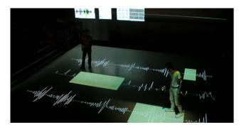
Audiodome Playground – A walkable  $8\times 8m$  floor projection, combined with an  $8\times 3m$  wall projection form the board of Audiodome Playground. The players interact using modified Wii controllers that have been integrated in the tracking system of the Animax.
